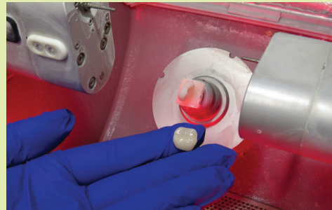
CEREC in-office custom crown milling machine makes a permanent crown in the time it used to take to make a temporary one!
